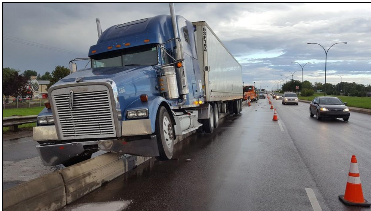
Figure 1-2: An eastbound tractor-trailer got hung-up on the low-profile barriers – conditions at the time were early morning (dark) and rain. Photo credit: Global Saskatoon, August 17, 2016
