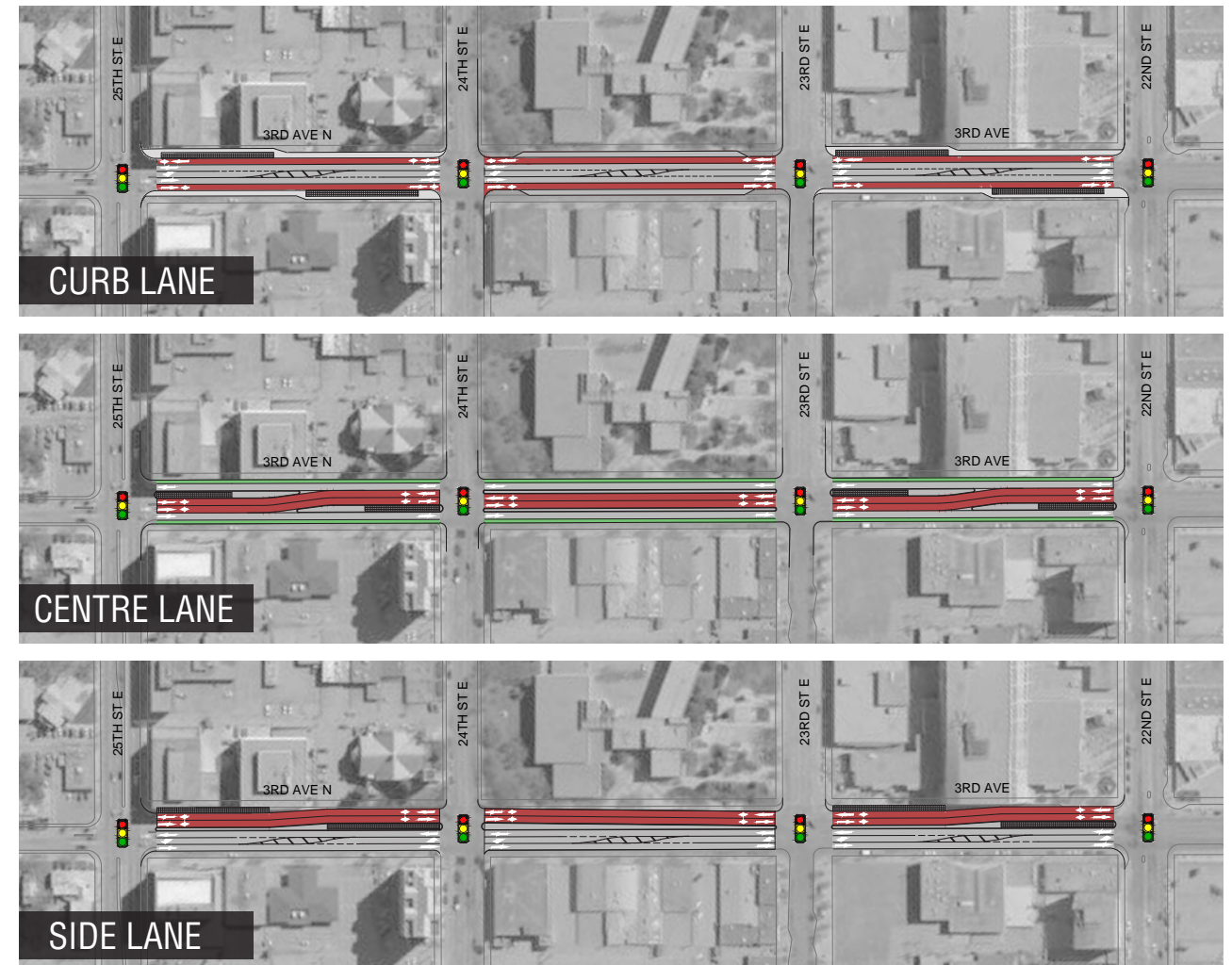
Figure 3.36 - Alternative BRT Configurations for 3 rd Avenue
