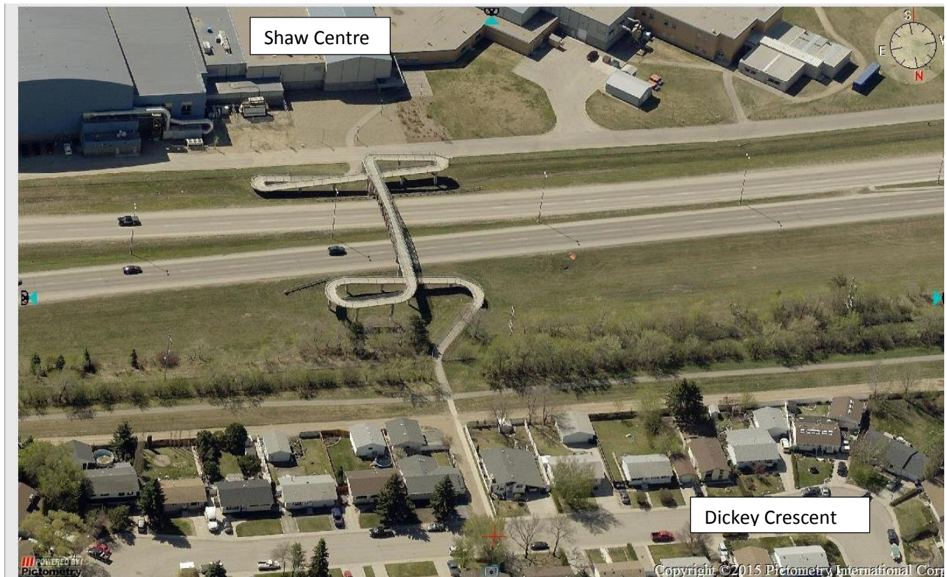
Figure 2: Path from Dickey Crescent to Shaw Centre over 22 nd Street West showing back lanes, berm, and pedestrian overpass.
