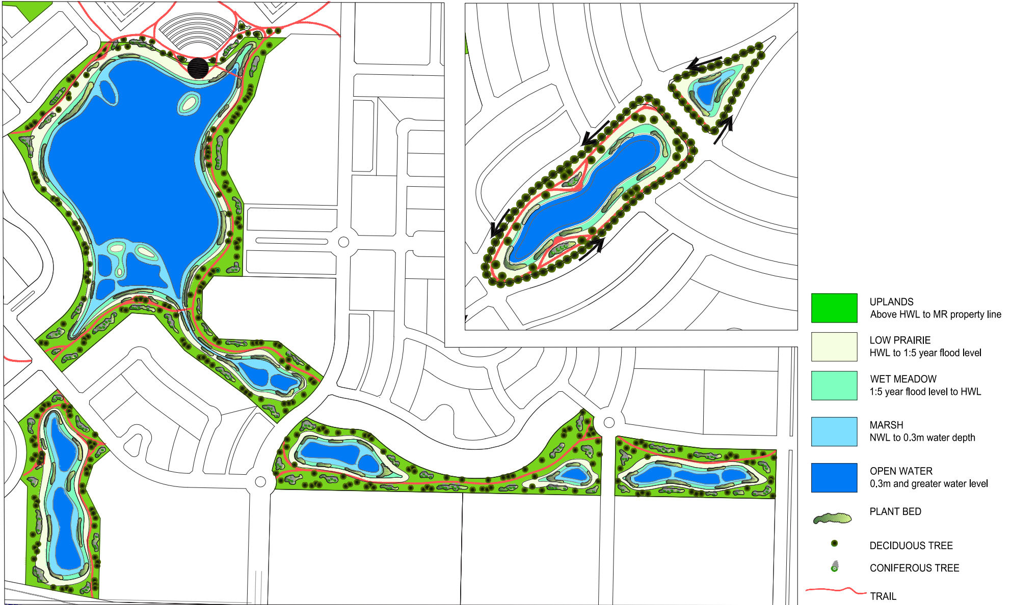
Figure 19: Constructed Wetlands Complex/Stormwater Facility Plan
