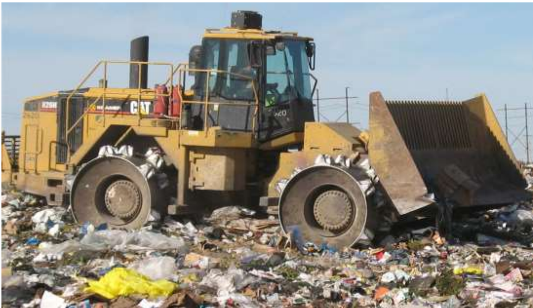
Compactor in operation at the Regional Landfill
