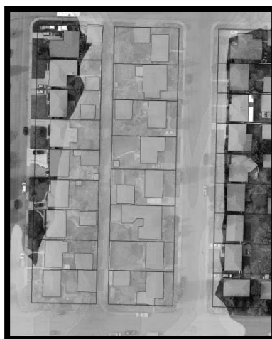
Figure 2: An example of flooded buildings during a 5 year storm.
