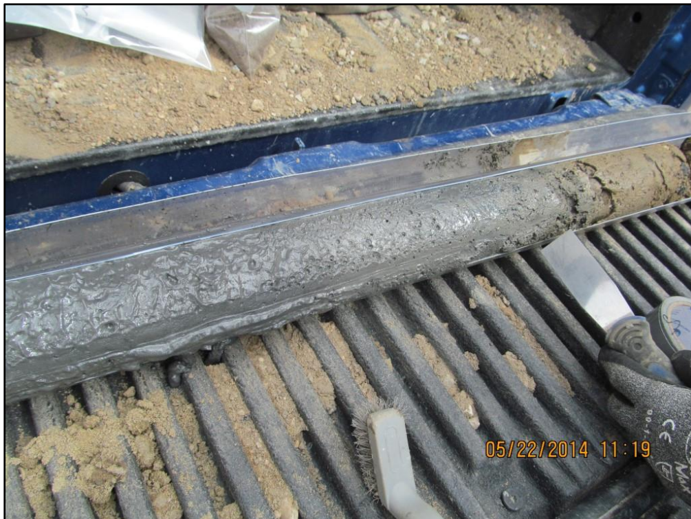
Photograph #8: Soil core removed from borehole 14-24. This soil core had a strong hydrocarbon odour. Note the staining.
