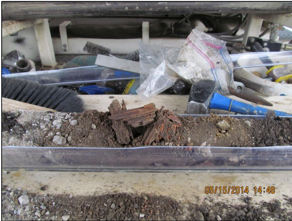
Photograph #5: Soil core from borehole drilled into historic mechanic's pit in storage yard of 321 Avenue C North. Note the wood and concrete.
