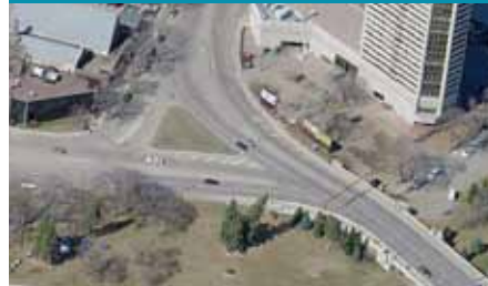
4.20 Channelized turn lanes on 19th St. and 4th Ave.
