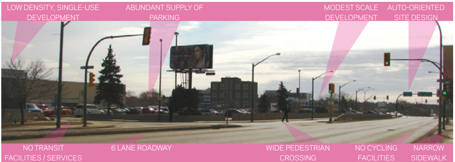
Figure 2.4: Idylwyld Drive - An Auto-Oriented Corridor
