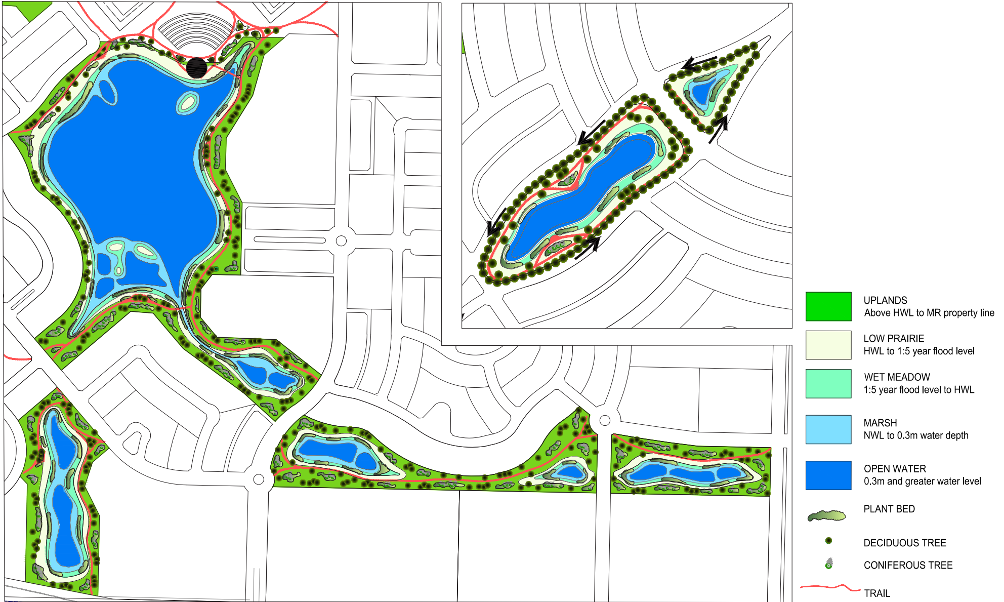
Figure 19: Constructed Wetlands Complex/Stormwater Facility Plan
