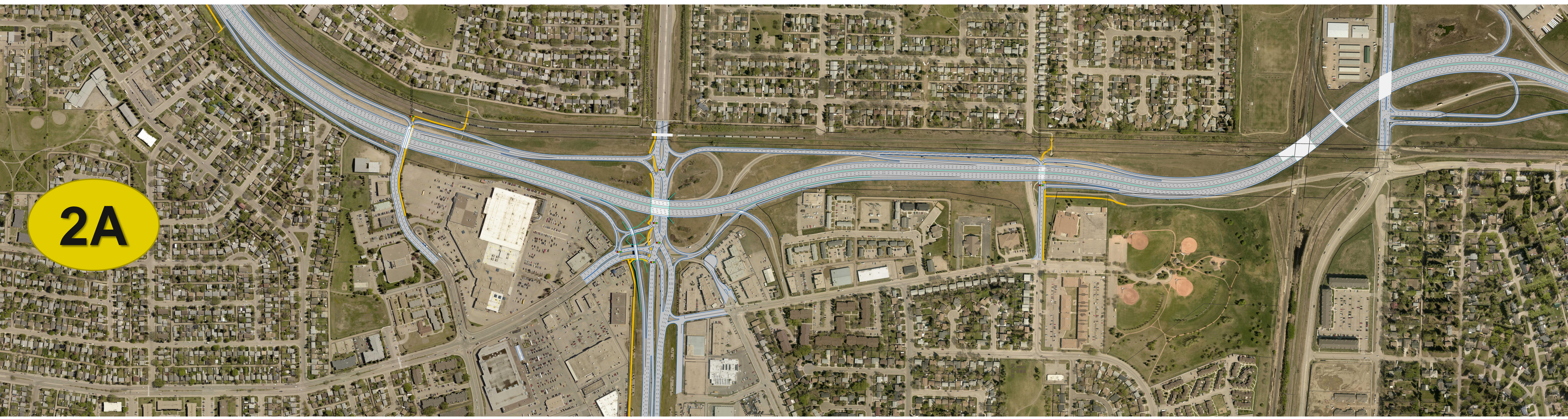
Diverging Diamond Interchange (DDI); with enhanced southbound C/D road connections passing Clancy Drive; and with Partial Interchanges at Laurier and Clancy Drives
