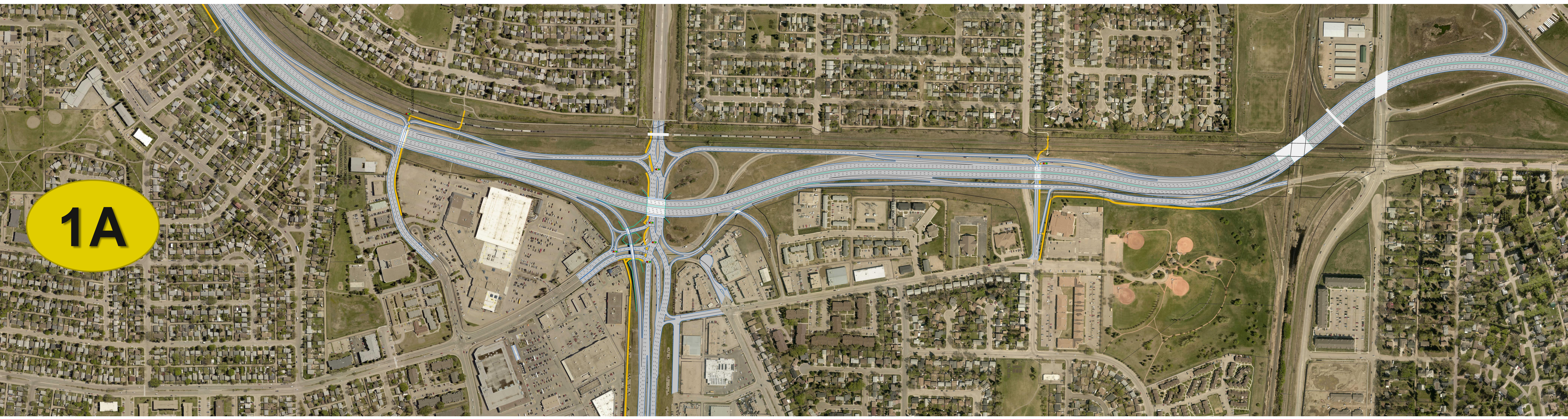
Diverging Diamond Interchange (DDI); with partial C/D Roads; and with Partial Interchanges at Laurier and Clancy Drives
