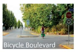
Bicycle Boulevard: these facilities are also located on the street but include traffic calming measures to reduce vehicle operating speeds to 30 km/h or less allowing bikes to safely travel with vehicle traffic on quiet streets. Saskatoon has six kilometers of Bike Boulevard.
